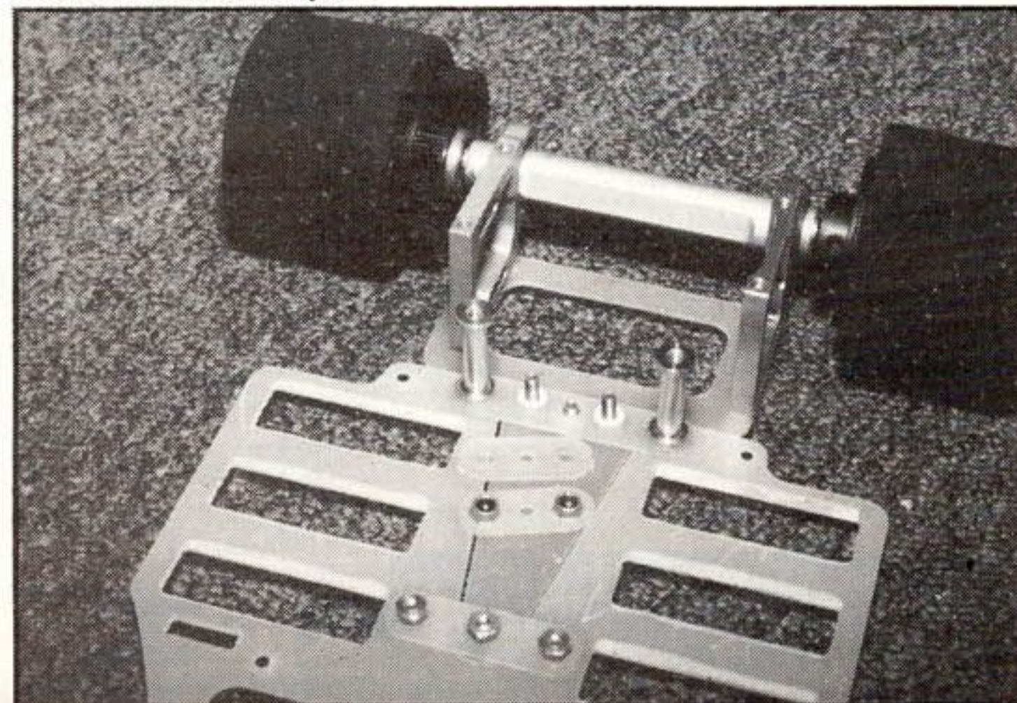
RC12L, with the supplied front suspension block support back in place with also an aluminium bracket in an attempt to keep the rear of the blocks apart.
